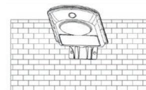
**GB** Possibility of wall or pole mounting via the supplied bracket
